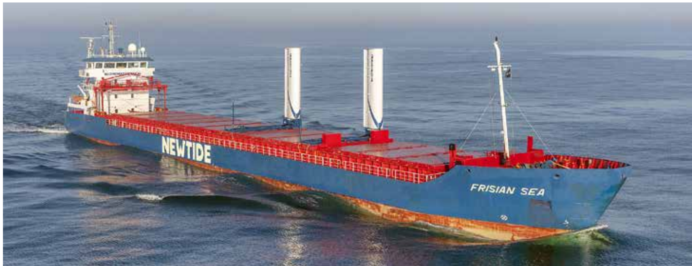
Flatrack Ventifoil unit from Econowind (courtesy Econowind).
