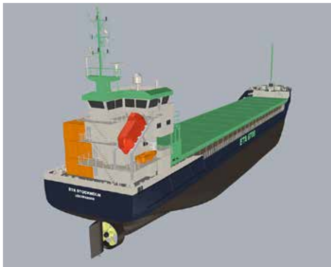
Aft deck with place for machinery/power plant containers and the propeller with nozzle and rudder (courtesy ÈTA Transitions).
